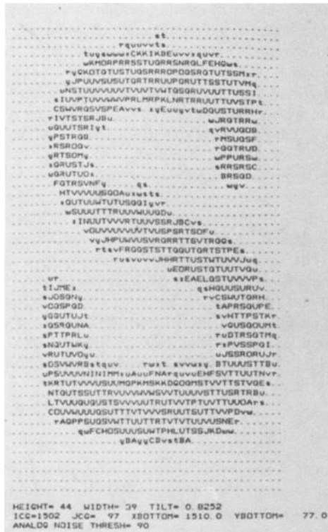
FIG. 2—A computer printout of a single character. The arrows indicate areas where the random effect of the ribbon and paper occur. The letters which make up the character represent gray scale with darker areas indicated by uppercase letters higher in the alphabet.
